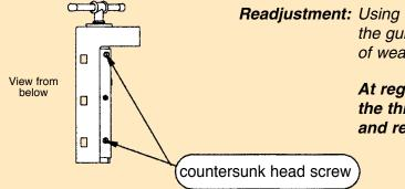
**Readjustment:** Using two countersunk screws on the underneath, the guide can be readjusted depending on the degree of wear to restore freedom from backlash.
