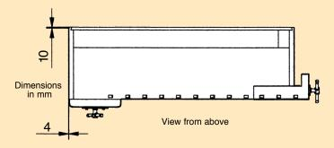
The bench top is permanently fixed to the trestle using four 6x80 countersunk head Spax screws. Drill holes have been prepared for this in the factory on the underneath of the bench top. To assemble, simply place the bench top on the trestle, align the top as shown in the sketch on the left and screw four countersunk head Spax screws into the top from below.
