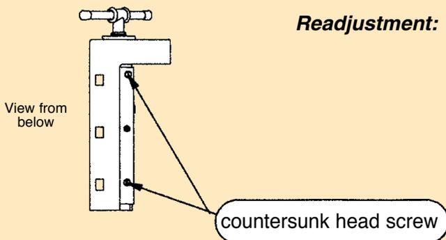
**Readjustment:** Using two countersunk screws on the underneath, the guide can be readjusted depending on the degree of wear to restore freedom from backlash.
