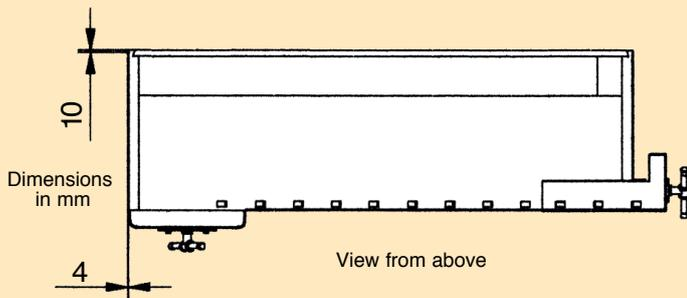
The bench top is permanently fixed to the trestle using four 6x80 countersunk head Spax screws. Drill holes have been prepared for this in the factory on the underneath of the bench top.
